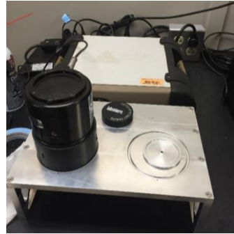
Visible and near infrared spectroscopy (400 – 2500 nm)
